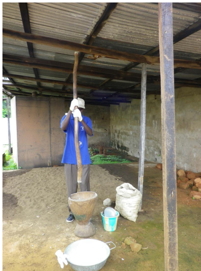
A wooden mortar was used to grain the oyster Shell
