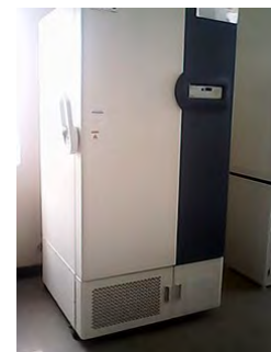
Image 5: Ultra freezer for long storage facility
