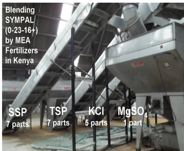
Figure 6: The MEA blending facility produces SYMPAL. SYMPAL (0-23-16+), composed of 7 parts TSP, 7 parts SSP, 5 parts KCl and one part MgSO 4 . Sympal is available in 2, 10 and 50 kg bags for about $0.79 per kg and is stocked by members of the Kenya Agro-dealers
