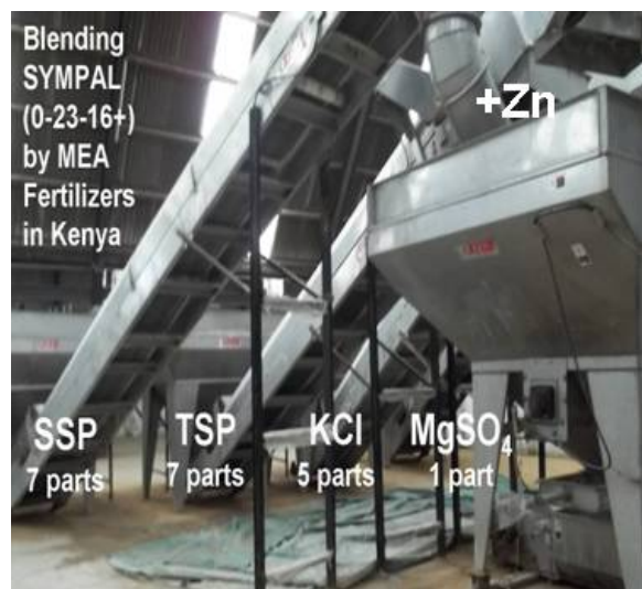
Figure 4.4: Fertilizer blending of Sympal at the MEA Ltd. factory in Nakuru, Kenya.
