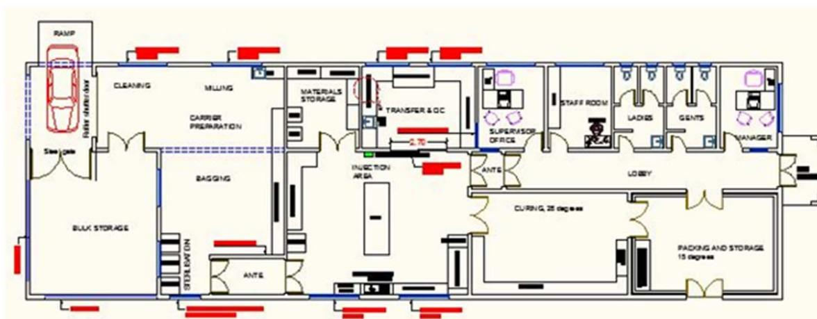
Figure 5.4: Floor plan of the inoculant factory under construction at IITA, Nigeria
