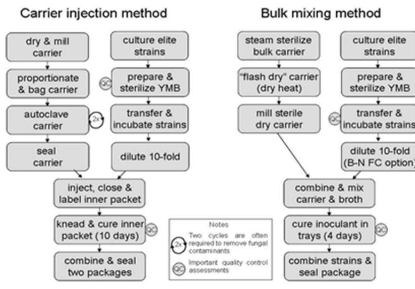
Figure 3.1: Comparison of the carrier injection and bulk mixing inoculant production processes
