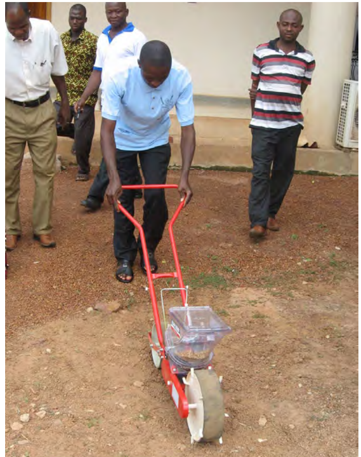
Testing whether a simple planter could sow inoculated seed without removing the inoculants from the seed surface
